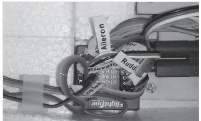
Insert each servo cable into its corresponding slot on the control board. Test and verify correct function of all control surfaces. After connecting all the servo cables, attach the control board in the location as shown above.
